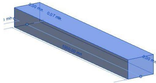
All beams may be modeled as a square/rectangular profile to represent the overall size of the beam only.
