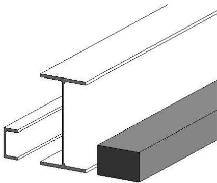
Beams will be modeled as their true profile type and will be modeled to the nearest 1/4" in size.
