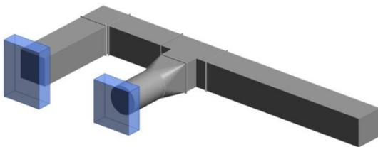
Ducting will be modeled using the standard MEP system tools within Revit. They will be modeled as a default duct type only. No system types will be indicated and fittings will be representative only. Any Pipe Accessories will be modeled as basic block forms indicating overall size and position only. All ducting sizes will be modeled.
