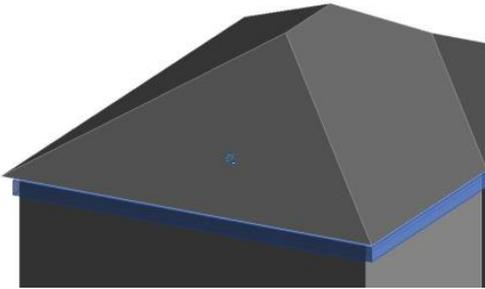
Detailing which extrudes from the host surface by over 8" will be modeled. It will be modeled as a basic block or simplified profile only.
