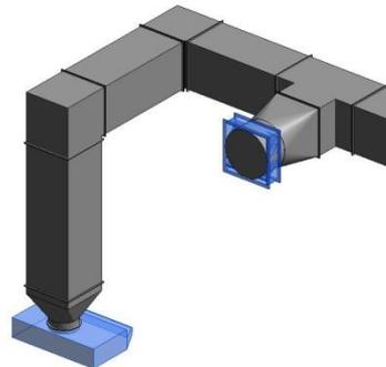
As in LOD 300 however all fittings and accessories will be modeled accurately. All sizes of ducting will be modeled. ***If service types are required then third party information would need to be supplied by the client. This would increase modeling time significantly.***
