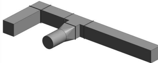
Ducting will be modeled using the standard MEP system tools in Revit. They will be modeled as a default type only. No system types will be indicated and fittings will be representative only. Only ducting over 6" will be modeled.
