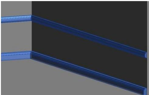
Detailing will be modeled where it extrudes more than 2" from the host surface and will be modeled accurate to its true profile.
