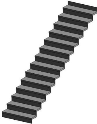
Stairs will be shown as a generic type with the correct number of treads and risers shown. No railings or stringers will be modeled.
