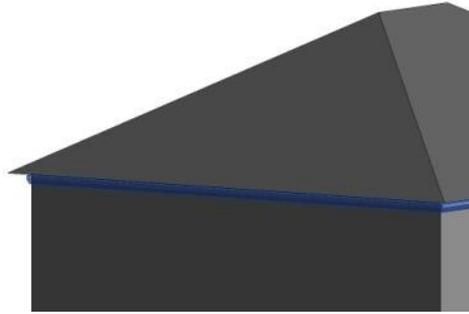
Detailing will be shown where it extrudes by more than 4" from the host surface. It will be modeled to represent the general profile shape of the profile in a simplified profile.
