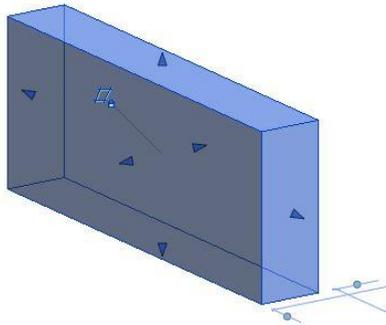
Beams may be modeled as basic model in-place extrusions categorized as Ceiling. Multiple elements may be modeled as one in-place family such as a group of rafters.
